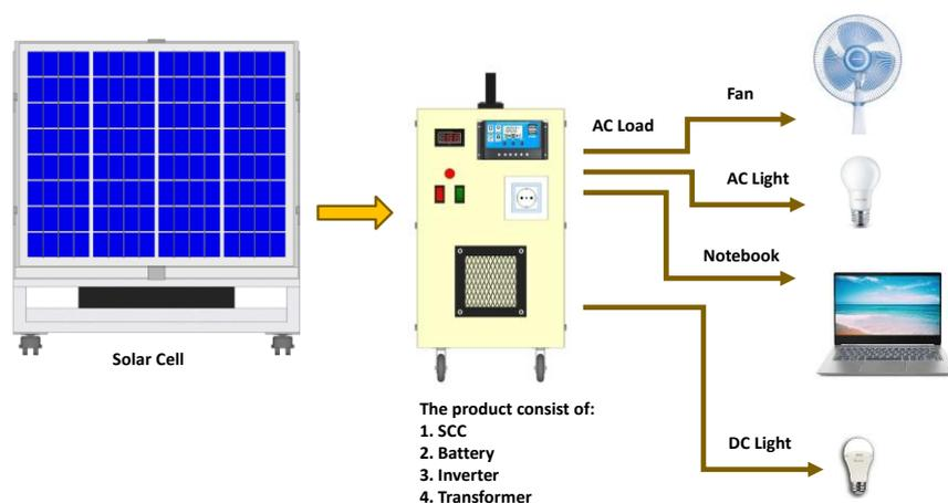
Figure 1. Schematic of the battery charging device
