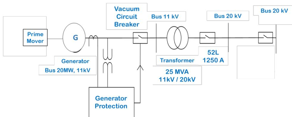
Figure 2. Single line diagram of Gas Power Plant at Riau Power
