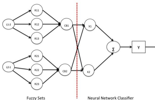
Figure 6. Structure of Fuzzy Neural Network Classifier
