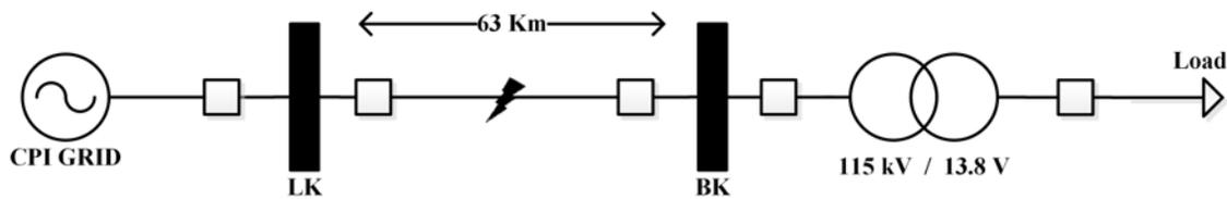
Fig. 4. Single line diagram transmission system
