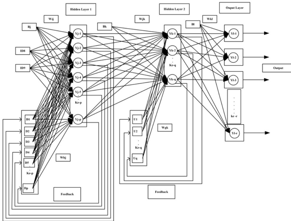
Figure 5. Elman’s RNN Structure of fault classification
