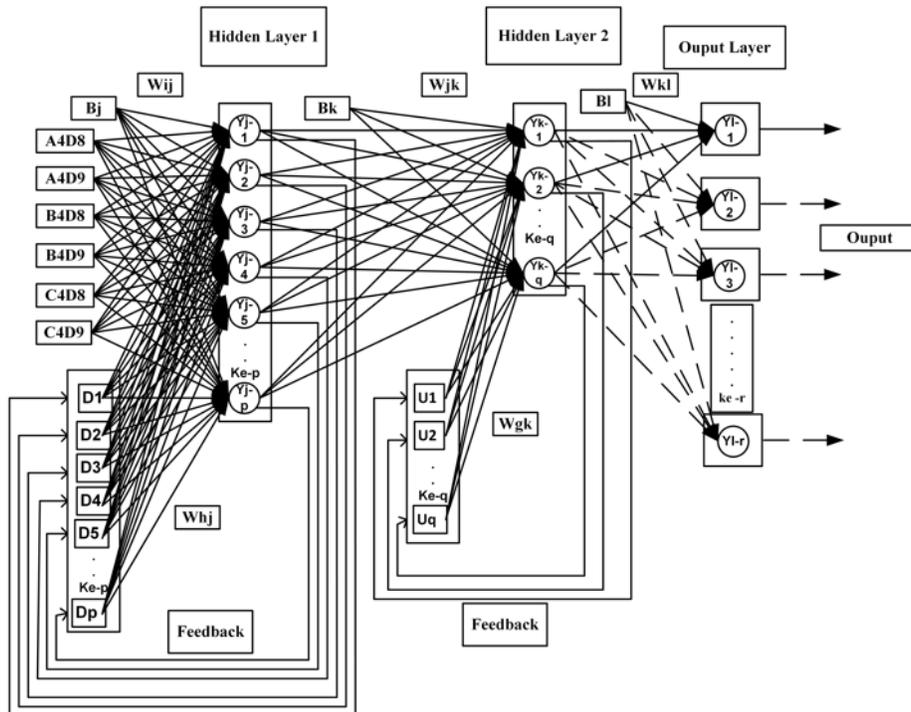
Figure 6. Elman RNN structure estimated fault location
