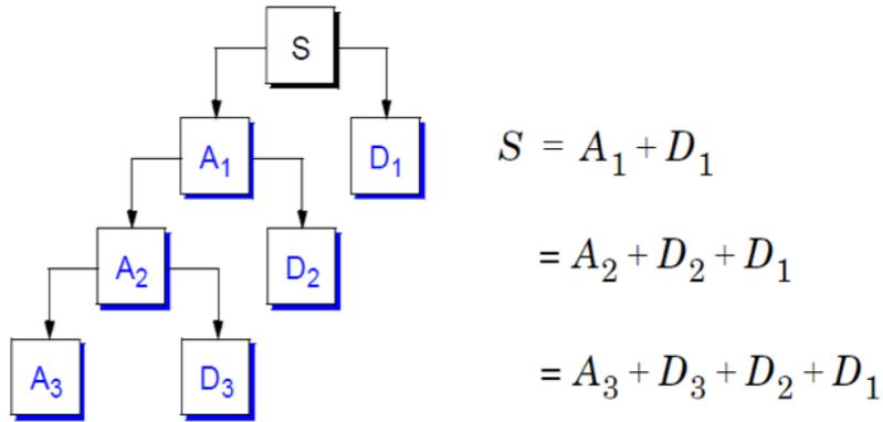
Fig. 2. The iteration is DWT decomposition
