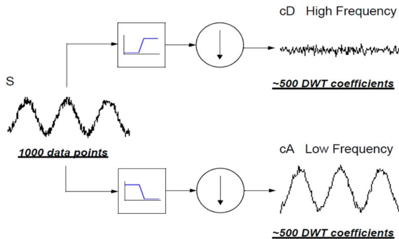
Fig. 1. Diagram signal processing DWT
