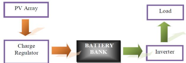
Figure 4: Scheme of the Battery charge and load system.
