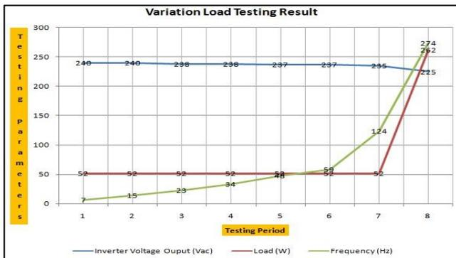
Figure 5: Frequency and voltage changing on variation loads.
