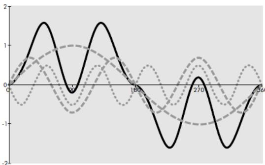
Figure 2: Current harmonic distortion.
