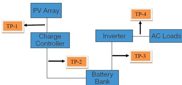
Figure 3: SEPG power quality of testing points.
