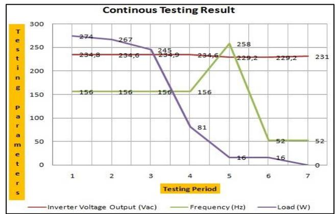
Figure 6: Frequency and voltage changing on continuous loads
